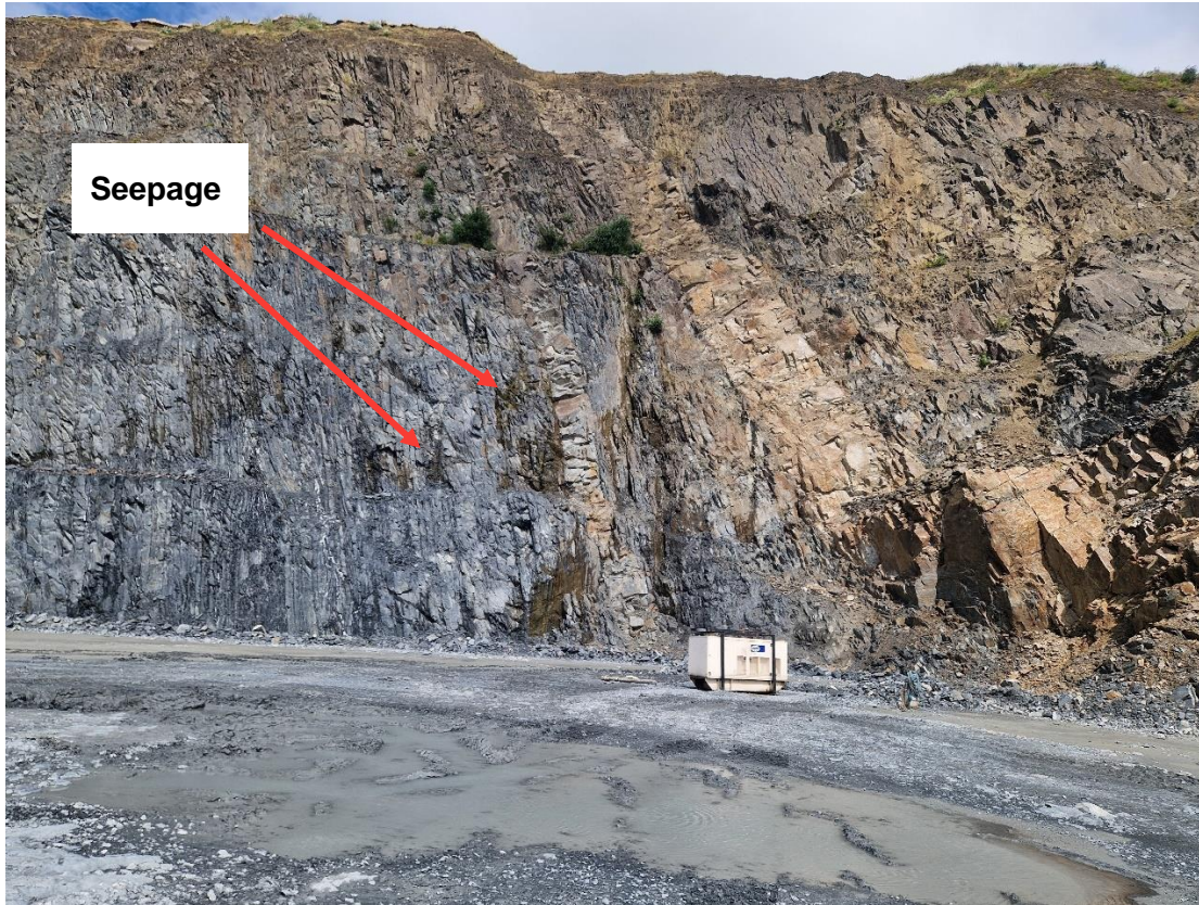
Figure 6-2 - Eastern Wall Seepages
