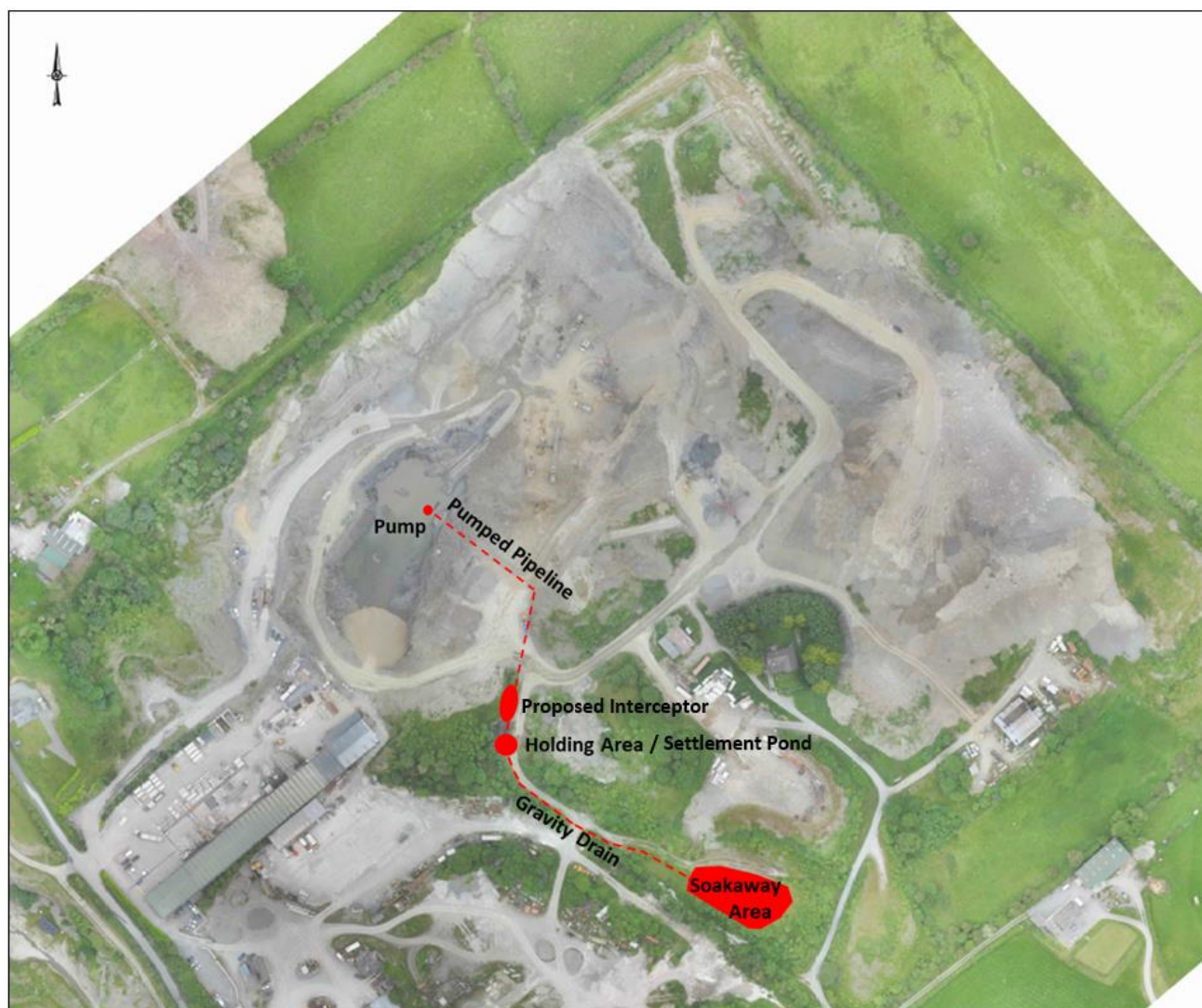
Figure 6-9: Layout of December 2019 dewatering and discharge system
